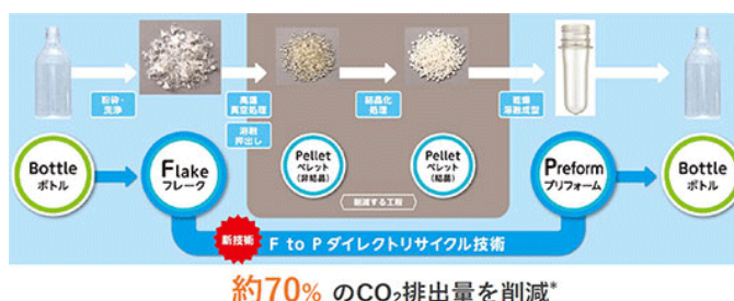
F-to-P direct recycling technology process
