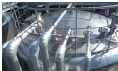
Reuse of water recycled at each stage of cleaning stored in 200 ton tanks
