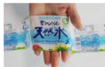
Roll label made with recycled PET bottles
