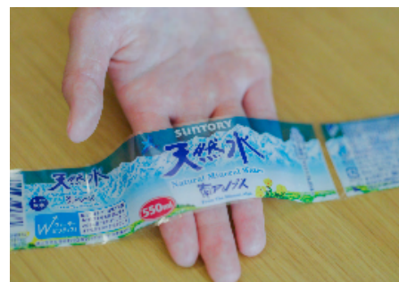
Japan's thinnest roll label at 12 \mu\text{m} thickness
